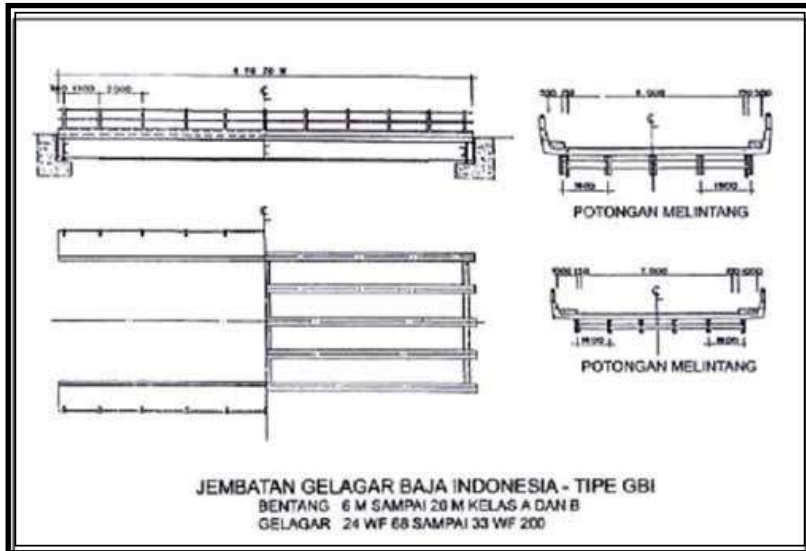
Gambar 8.15–Gelagar Baja Indonesia Tipe GBI Standar Sumber: https://thamrinnst.files.wordpress.com/2012/04/modul-6-sesi-5-jembatan-komposit-2016.pdf
