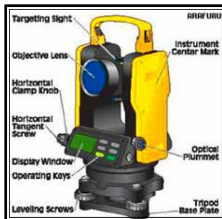
Gambar 10.4. Bagian-bagian theodolit
